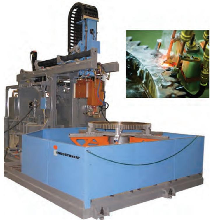
Figure 7. Example of Inductoheat's standard induction machine for tooth-by-tooth hardening large gears. (Courtesy: Inductoheat).
