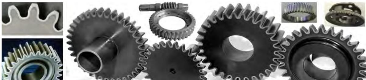
Figure 1. External spur and helical gears, worm gears, internal gears, racks, and sprockets are among those that are typically induction hardened.
