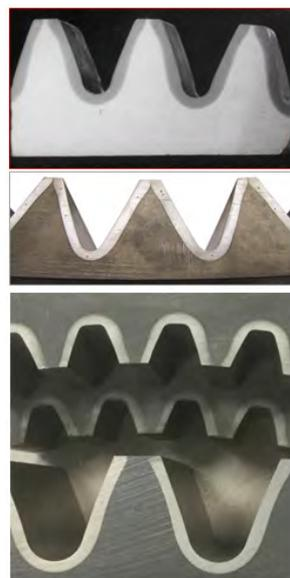
Figure 5. Examples of hardness patterns. (Courtesy: Inductoheat).
