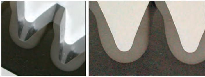
Figure 6. Example of undesirable softening of the areas adjacent to the hardened area (tempering back) [1].
