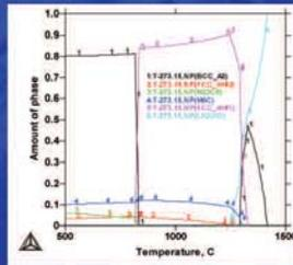
**DICTRA** is a unique software package for accurate simulations of diffusion controlled transformations.
