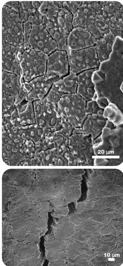
**Fig. 1** — Grain boundary liquation (top) and cracking (bottom).
