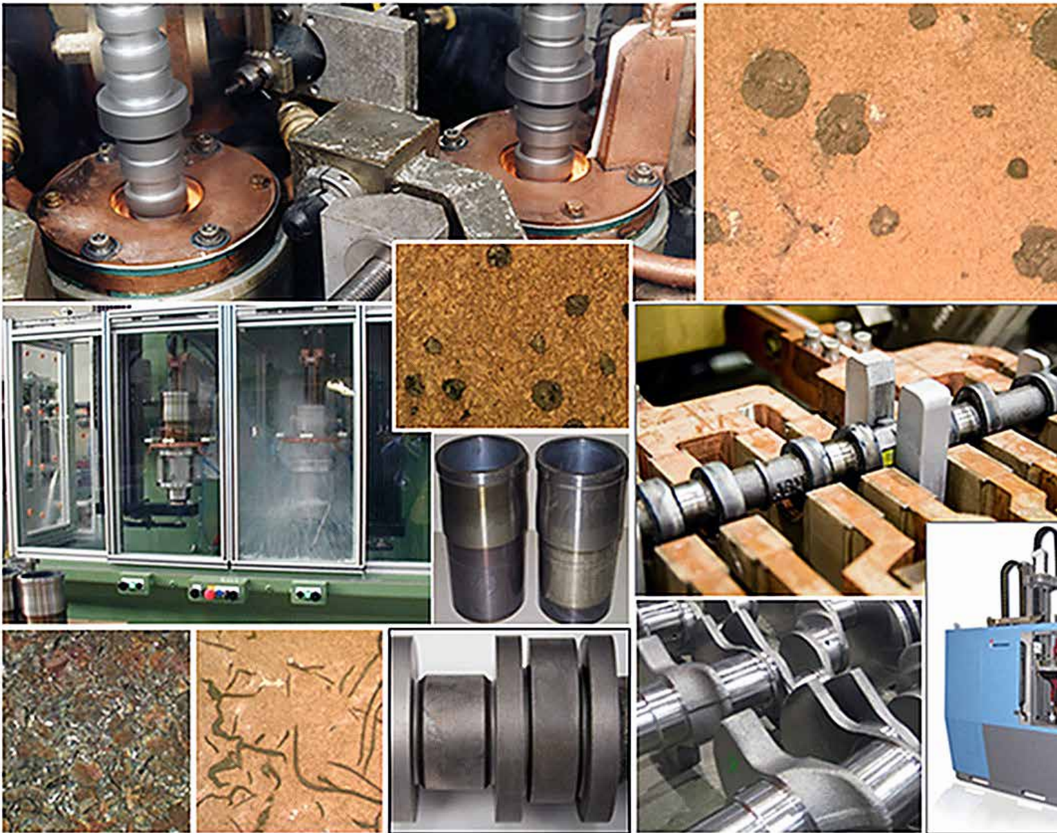
Figure 1: Induction heating is successfully applied for heat treating of a variety of iron castings offering numerous attractive properties, microstructures, and cost advantages for different commercial applications. (Courtesy: Inductoheat Inc., an Inductotherm Group company)
