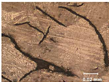
Figure 2: Ductile cast irons consist of graphite in shapes of spheroids or nodules (right). Graphite particles of gray irons appear in 2D metallographic examination in flake-like form (left) [1].
