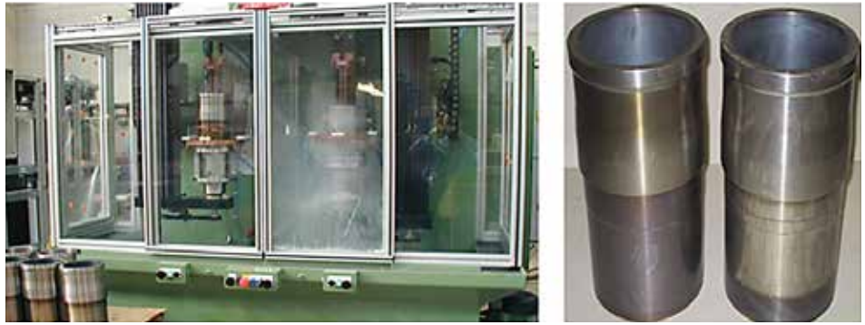
Figure 3: Unitized machine for IH of gray iron cylinder liners for commercial vehicle engines (Courtesy: Inductoheat Inc., an Inductotherm Group company).
