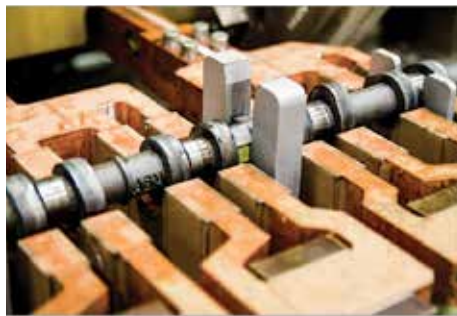
Figure 8: Close-up of Inductoheat’s SHarP-C inductor (a) and as-hardened microstructure (b) that reveals the two-phase (fine-grain martensite and nodular graphite) structure with an insignificant amount of retained austenite. (Courtesy of Inductoheat Inc., an Inductotherm Group company.)
