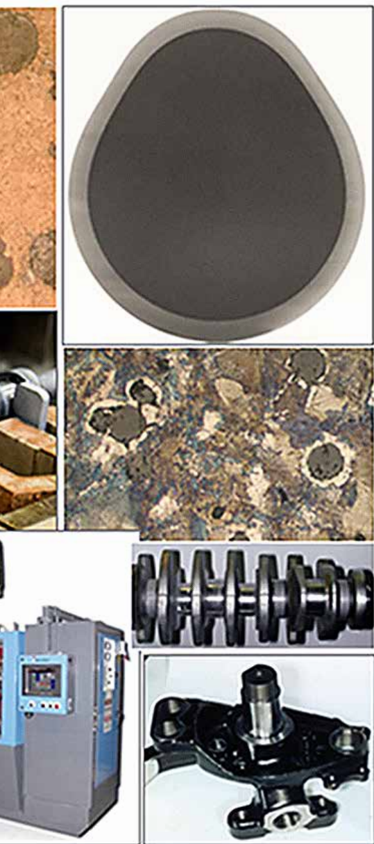
Figure 2: Ductile cast irons consist of graphite in shapes of spheroids or nodules (right). Graphite particles of gray irons appear in 2D metallographic examination in flake-like form (left) [1].
