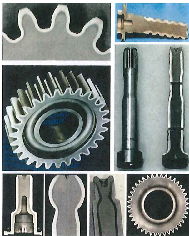
Fig. 2 — Induction heating enables heat generation in localized areas where metallurgical changes are desired.
