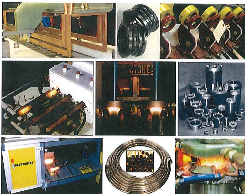
Fig. 1 — The highly controllable heat intensity of induction heating enables optimizing a wide variety of heating and hardening processes.
