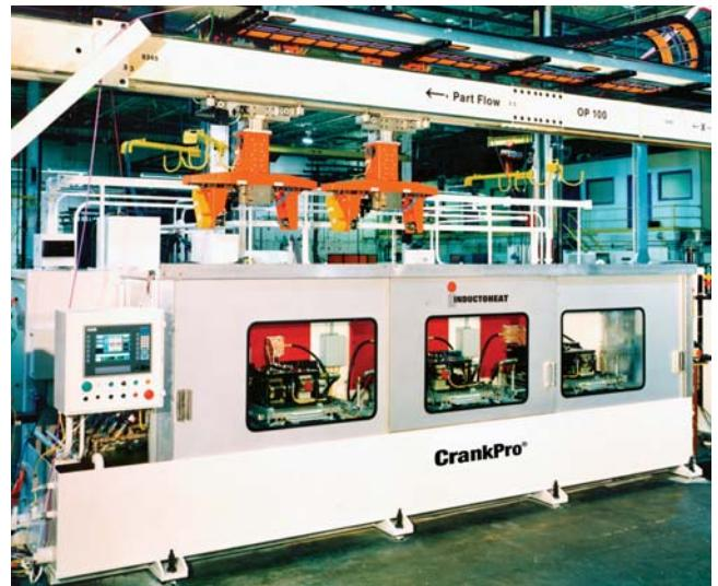
**Fig. 4.** CrankPro machine implements Inductoheat's patented non-rotational crankshaft hardening and tempering technology
