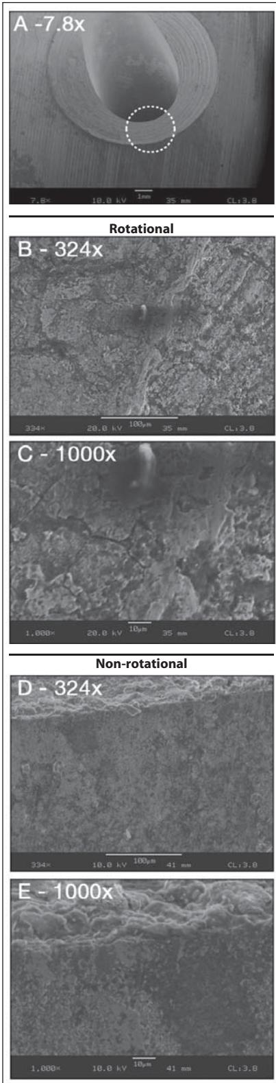
**Fig. 8. The results of SEM analysis of similar regions near oil hole using rotational and non-rotational technology. Note: There is indication of a grain-boundary liquation with rotational hardening process.**
