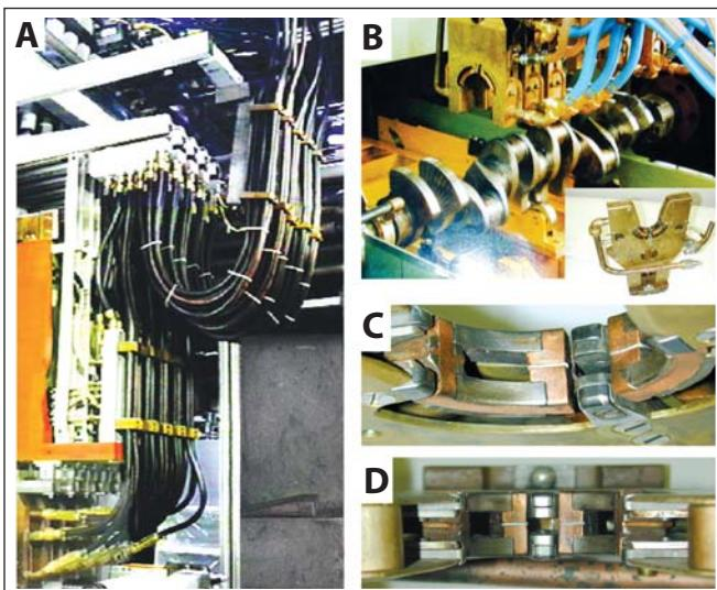
**Fig. 3.** Rotational hardening process utilizes a number of U-shaped inductors. Note: Carbide guides (locators) are required.
