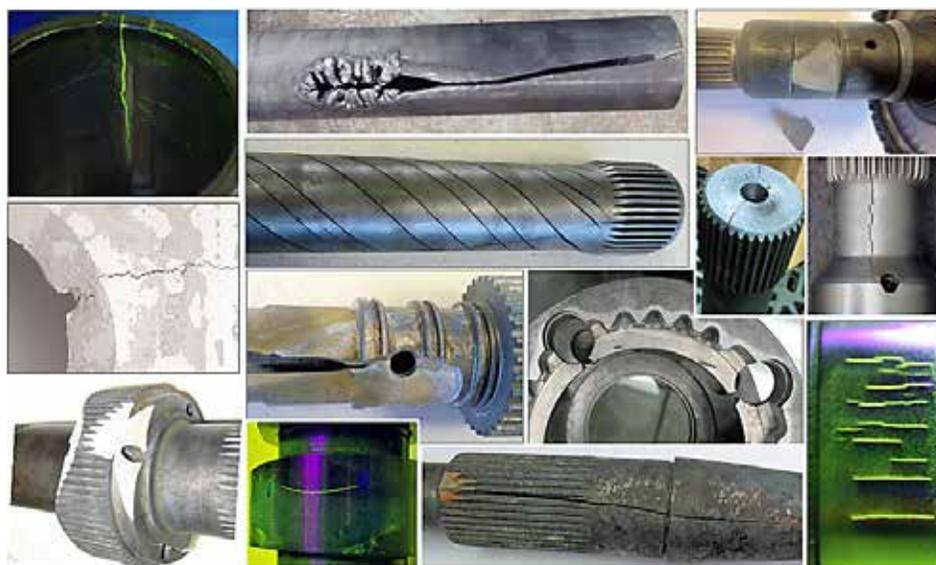
Figure 1: Examples of typical cracks caused by improper process recipes or inductor designs.
